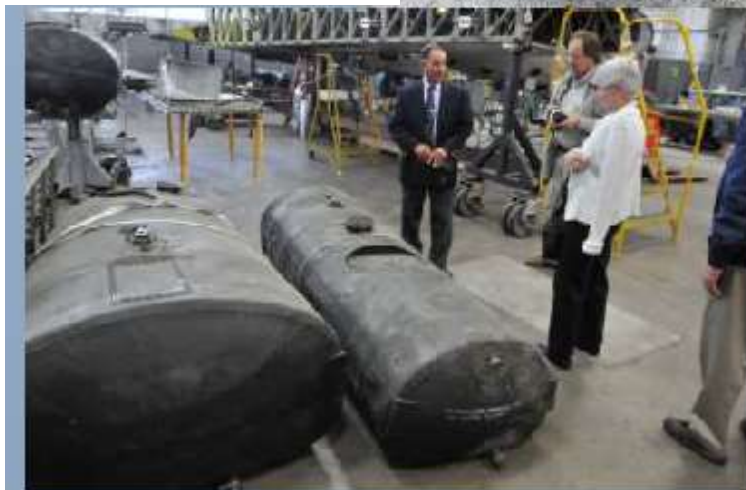
Bullet/puncture -proof rubber fuel tank (burnt remains)
