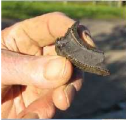
Bullet/puncture -proof rubber fuel tank (burnt remains)
