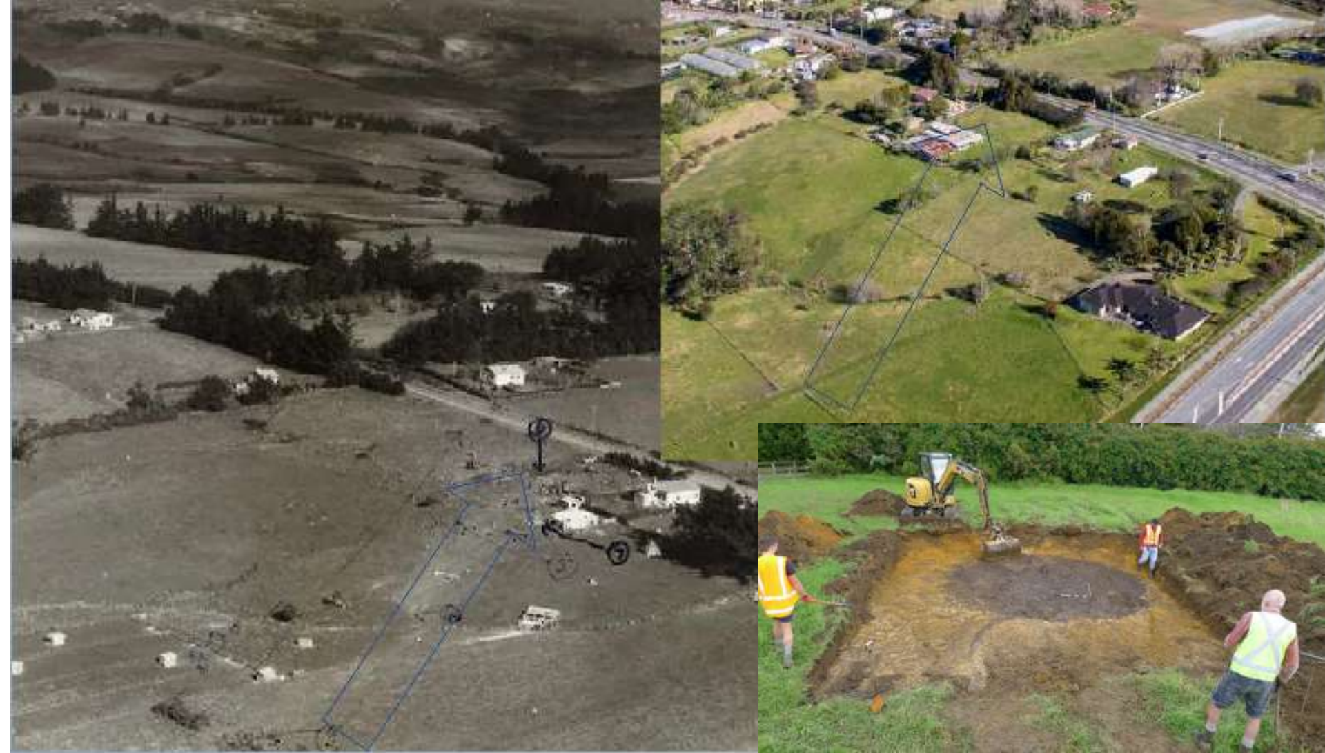
Infilled crater located by ortho-rectification of aerials, probing and test pitting
